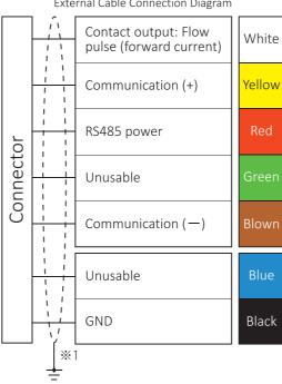
※1. The main body and GND are electrically common. Use an isolated power supply and indicator as required.
